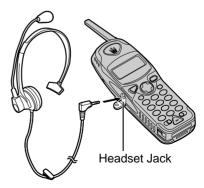
When the optional headset is connected to the cordless handset, make sure to use the headset to talk with the caller. If you want to have a normal cordless phone conversation, disconnect the headset.
