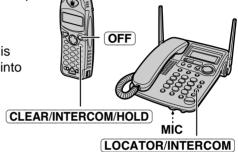
When using the handset, place the handset on the cradle. When using the speakerphone, press (LOCATOR/INTERCOM).
